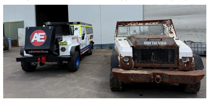
Another example of a Driftrunner (a vehicle used in underground mining) being refurbished.
